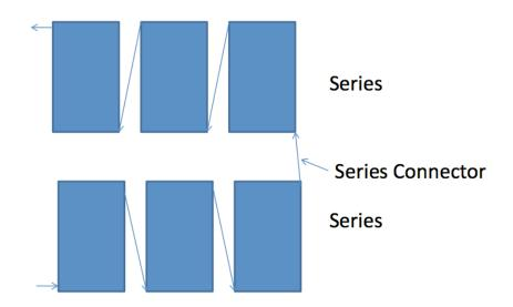
The number of collectors in series per flow path is six.
