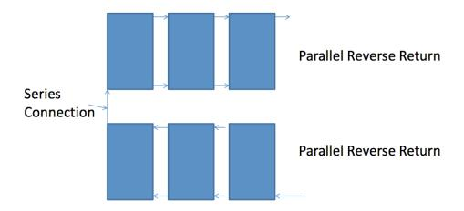
The number of collectors in series per flow path is **two.**
