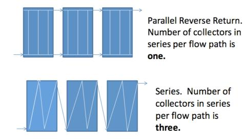
Note: The number in the flow path depends on how many times a drop of water is heated, i.e. it depends on the external piping configuration, not the internal piping configuration.
