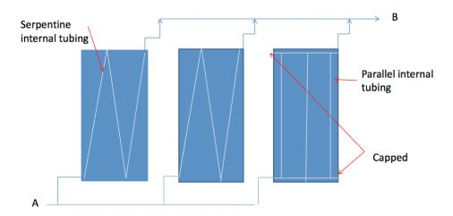
These collectors may have internal parallel piping or internal serpentine piping. Either way, the parallel external manifolds cause each molecule of water passing from A to B to flow through only one collector. The number of collectors in series per flow path is **one.**
