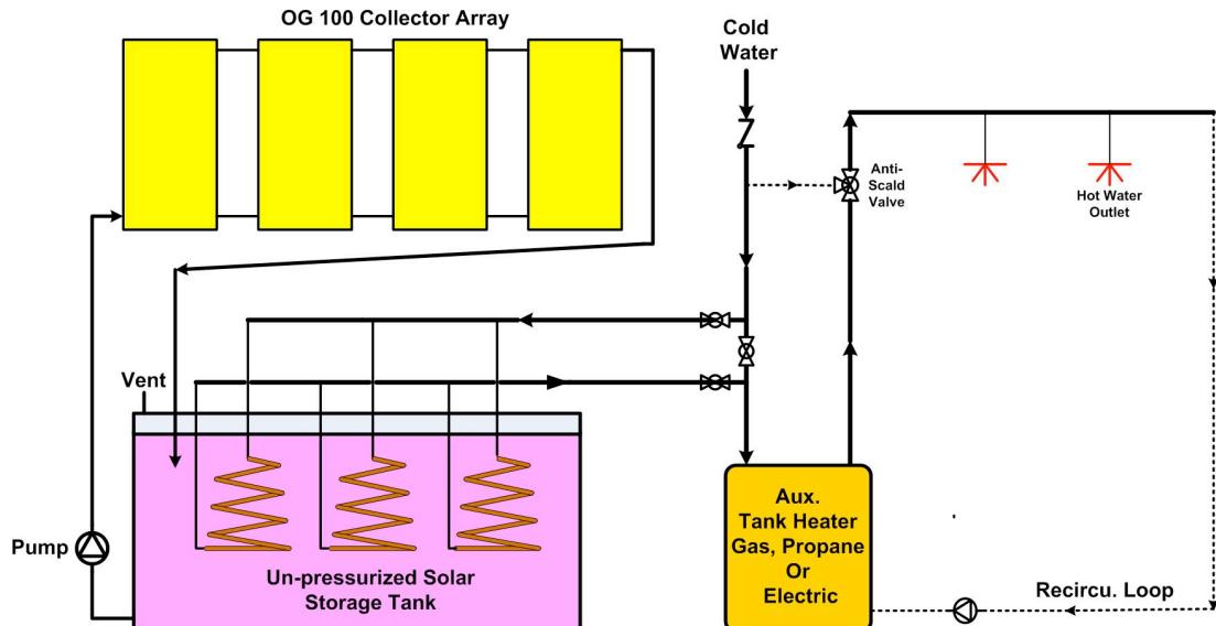
**Example B – External Supply Side HX Indirect Forced Circulation System with Tank-less Heater**
