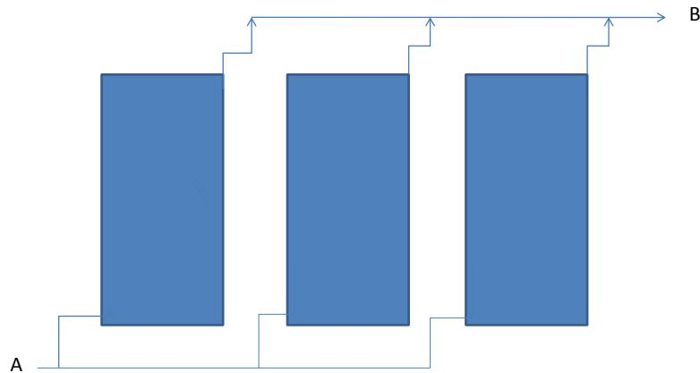
These collectors may have internal parallel piping or internal serpentine piping. Either way, the parallel external manifolds cause each molecule of water passing from A to B to flow through only one collector. The number of collectors in the flow path is **one**.
