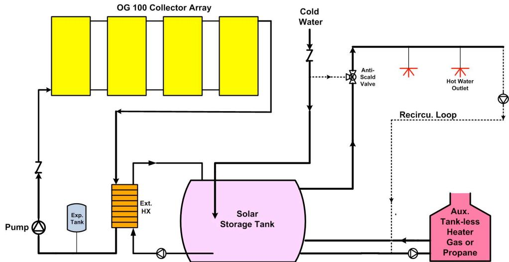
**Example C – Immersed Supply Side and Immersed Load Side HX IFC System with Tank Heater**
